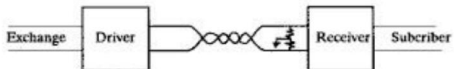
Fig.28: balanced circuit connection
